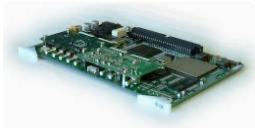
2002: HDTV Encoder (with VASA) Post-card-size / 15 W NHK•NTT Com
